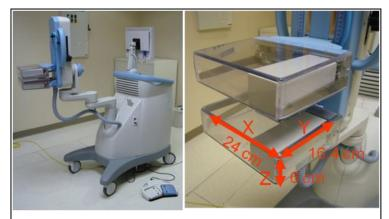
Figure 1.1: The Naviscan PEM Flex Solo II positron emission mammography scanner (Left). The detector heads inside the compression paddles (Right).
