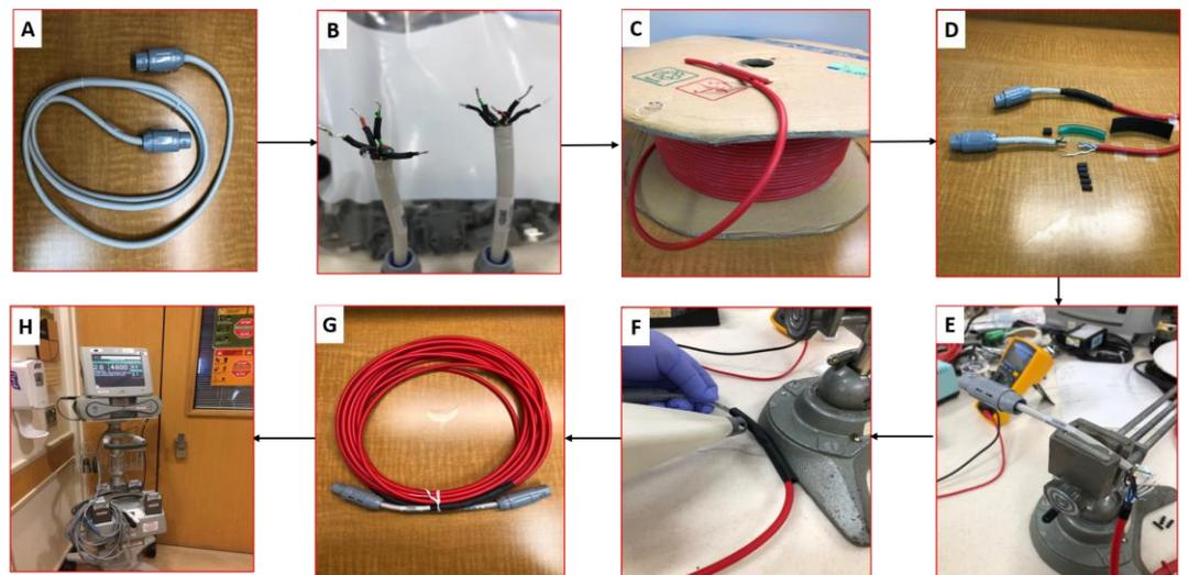
For the HeartWare HVAD system, we tested a 35-foot low voltage computer data cable and found that there was a loss of data transmission at a total of 45 feet. A DB9 serial extension cable was tested and we found it was able to maintain the signal for 45 feet. Importantly, it is readily available at most computer or electronic stores.
