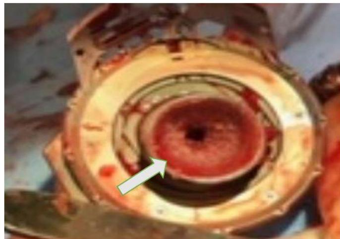
**Figure 2:** The arrow indicates the nearly occlusive thrombus in the HeartMate 3 left ventricular assist device system (Abbott Laboratories).
