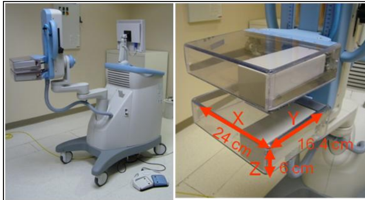
Figure 1.1: The Naviscan PEM Flex Solo II positron emission mammography scanner (Left). The detector heads inside the compression paddles (Right).
