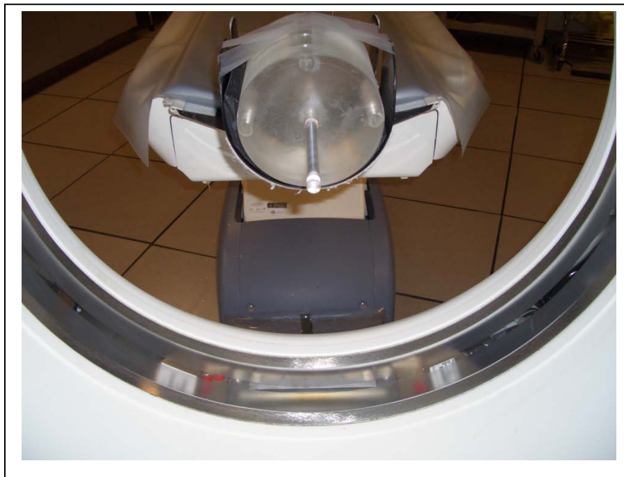
Figure 3-3. Configuration used to measure the unattenuated exposure ( I_0 ).
