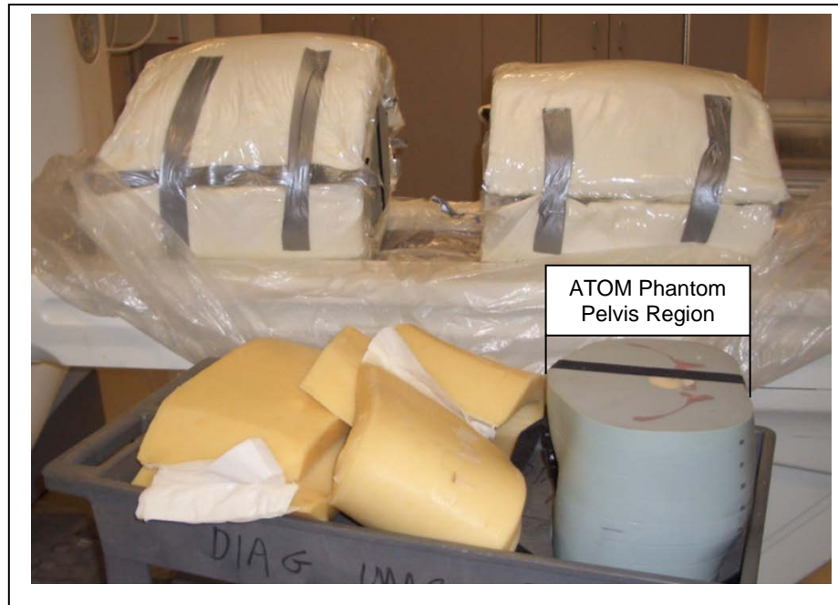
Figure 3-23. Disassembly of 99 th percentile phantom configuration for repeated TLD measurements during simulated VC; with the two layers of CIRS simulated phantom fat disattached from the ATOM phantom pelvis region (held in-tact during simulated VC by the black nylon strap shown).
