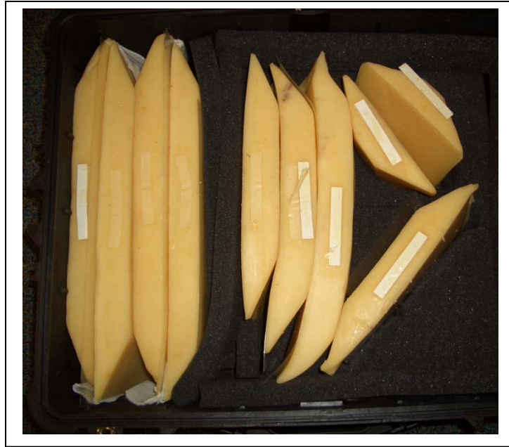
Figure 2-4. CIRS model 701 ATOM adult male phantom simulated adipose tissue kit.
