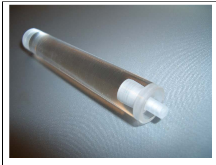
Figure 2-8. Female side of disassembled custom-made insert rod with TLD capsule placed in seating.
