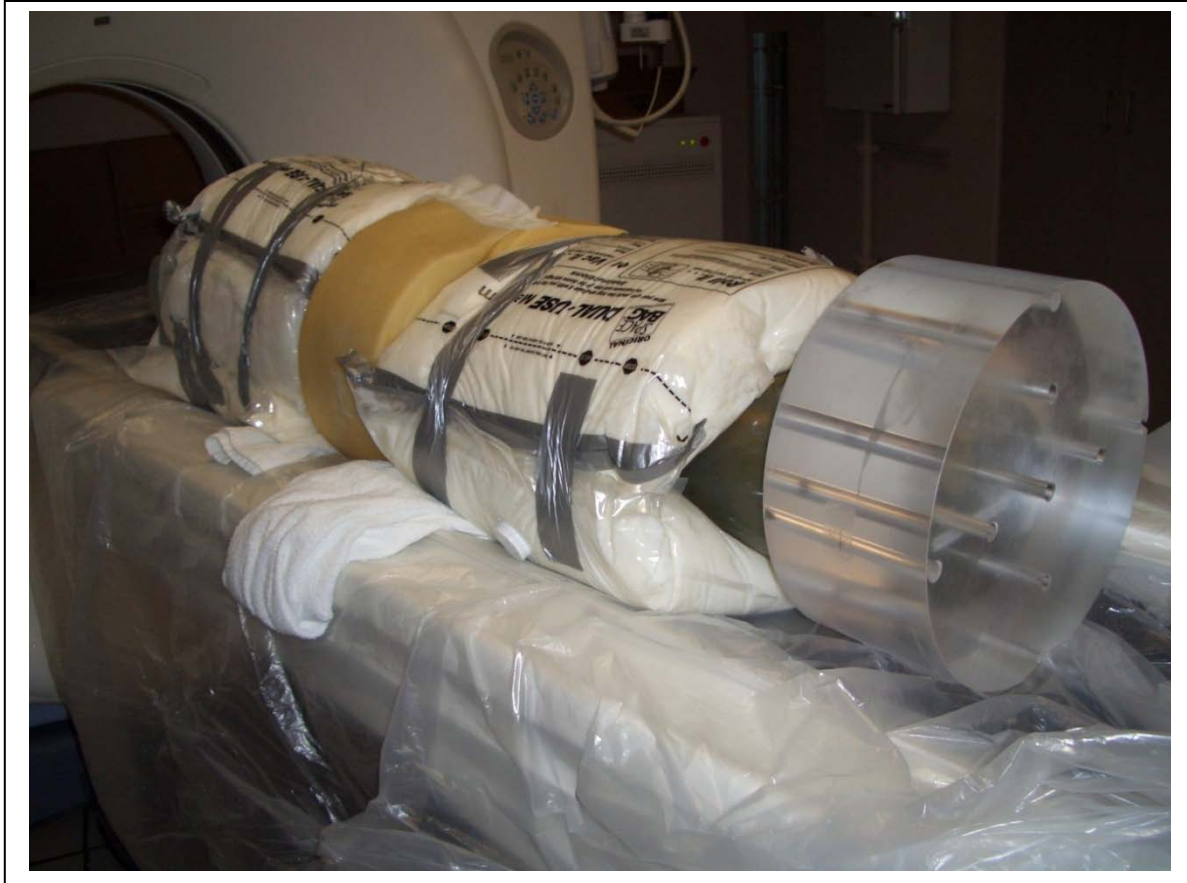
Figure 3-21. ATOM phantom assembled to represent the 87 th percentile of US adults aged 18-64 for simulated VC.
