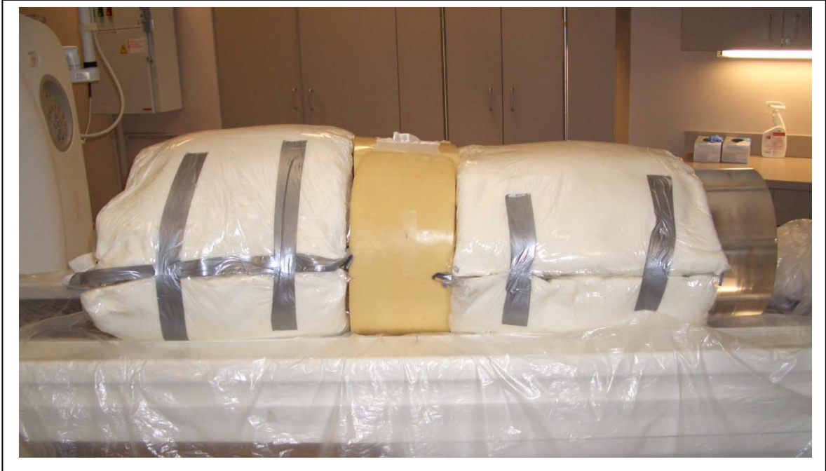
Figure 3-22. ATOM phantom assembled to represent the 99 th percentile of US adults aged 18-64 for simulated VC.
