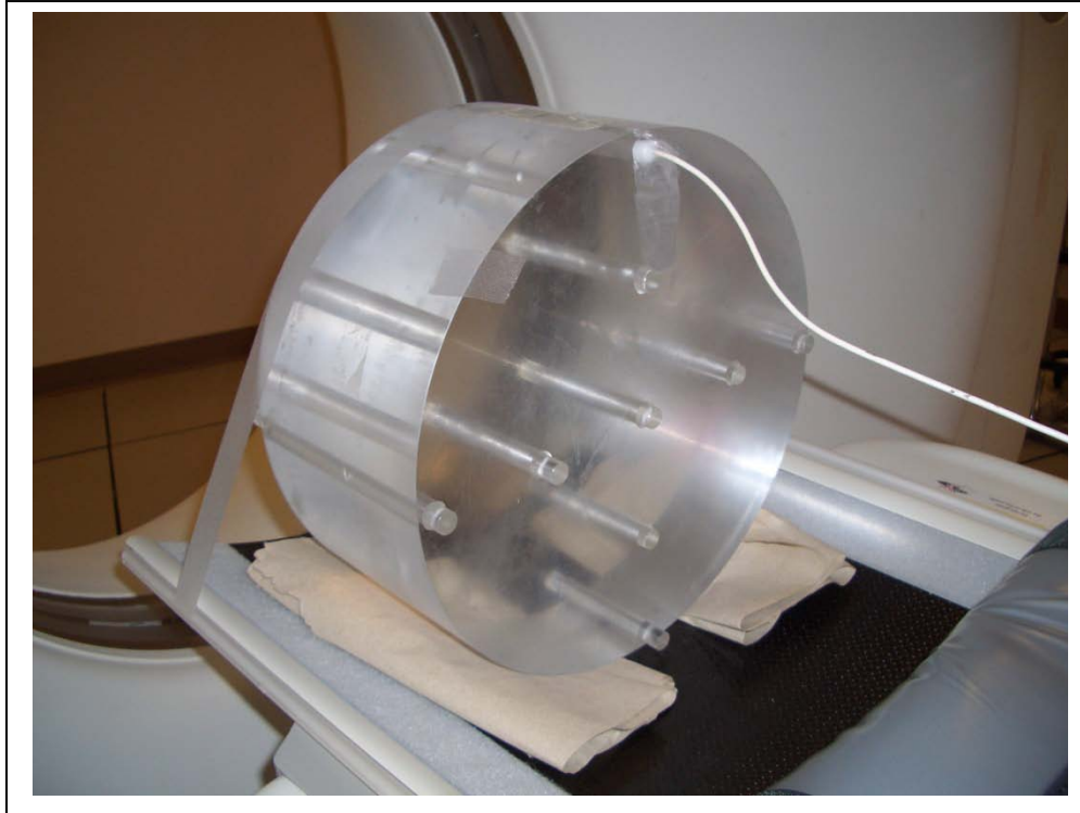
Figure 3-6. Configuration used to measure the exposure in the 12 o'clock bore of the CTDI body phantom, which was used to calculate (CTDI_{100})_{12} . A similar configuration was used to measure the respective exposures in the determination of (CTDI_{100})_3 , (CTDI_{100})_6 , and (CTDI_{100})_9 .
