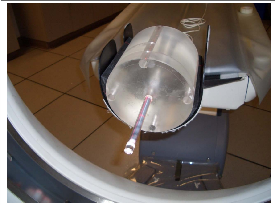
Figure 3-1. Using a CTDI head phantom on the head-holder attachment to place the pencil ionization chamber at isocenter of the CT scanner bore for in-air measurements.
