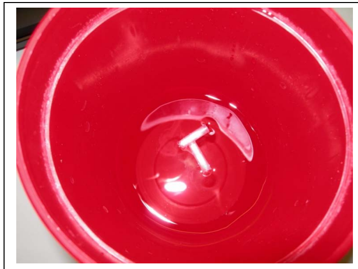
Figure 3-24. QA test #1: Place TLDs in a water bath for 24 hours.
