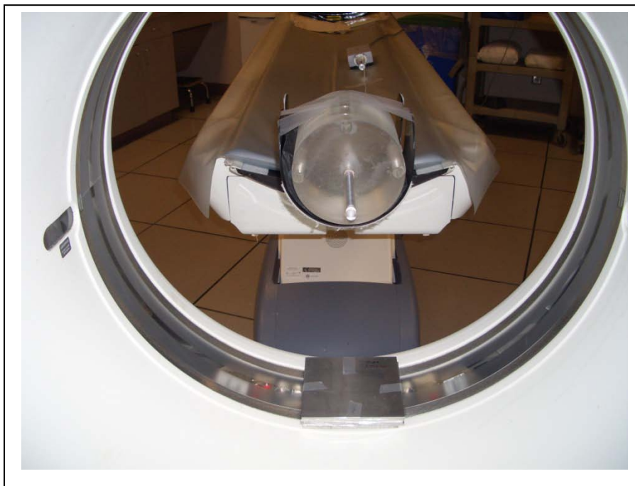
Figure 3-4. Configuration used to measure the x_1 and x_2 attenuated exposures ( I_1 and I_2 ).
