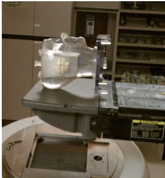
Figure 2.3 RPC IMRT Head and Neck phantom set up for irradiation on linac table
