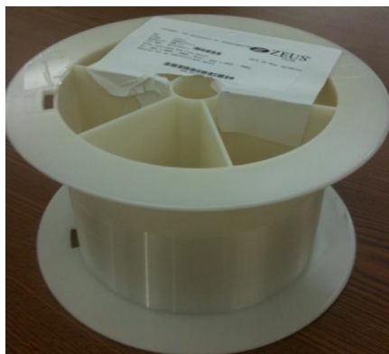
Fig.3.3: Hollow PTFE ultra-micro-bore tubing. Hollow plastic capillaries with smaller outer diameter than previously reported hollow plastic capillaries.
