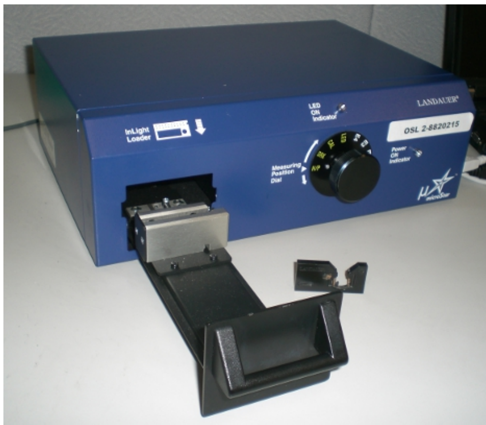
Figure 2.3: The microStar OSLD reader with tray pulled out. NanoDot OSLDs are read by inserting a single dosimeter into the black adapter jig pictured, then inserting the jig into the tray. The tray is pushed in and the knob turned to initiate the reading process.
