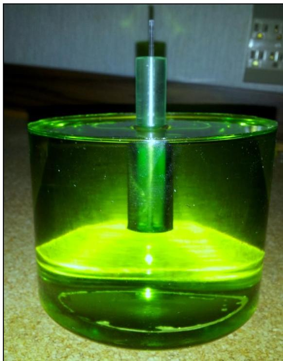
**Figure 15. Dosimeter with plug, catheter, and 6711 seed**
