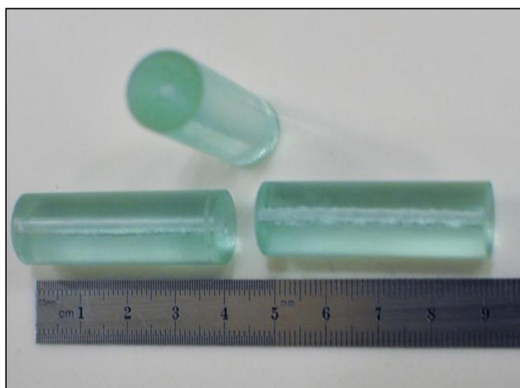
**Figure 10 PRESAGE® plugs for 1.5 cm diameter channels**
