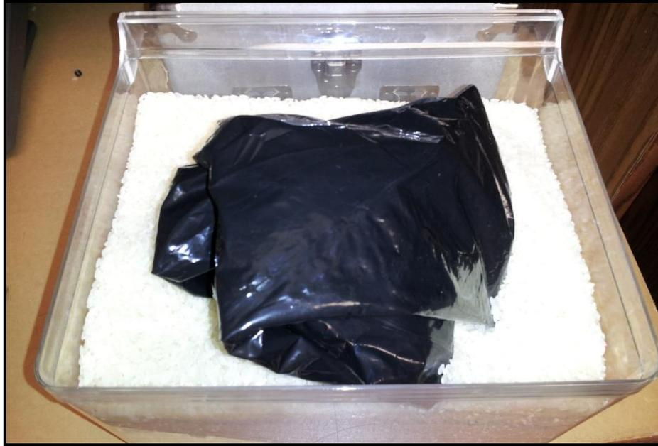
**Figure 14. Dosimeter (shielded from light) positioned in rice tank for backscatter**
