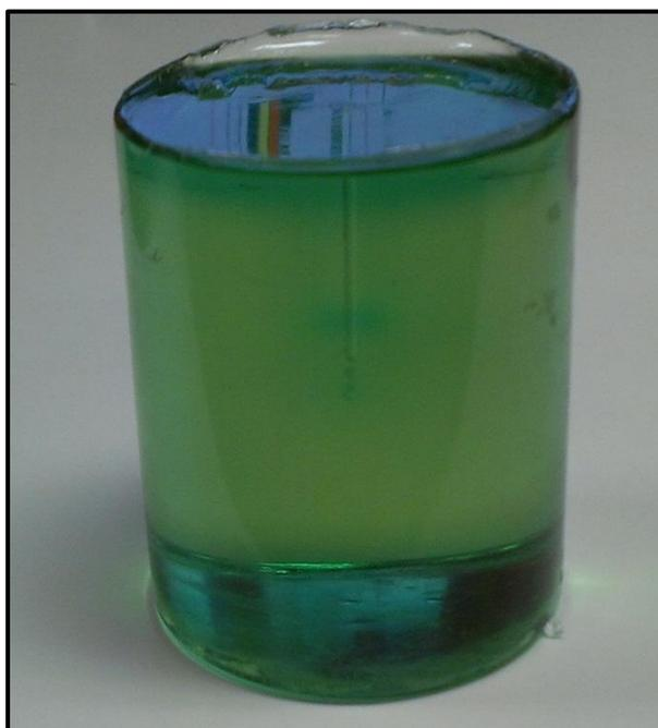
**Figure 3 Example of an irradiated PRESAGE<sup>®</sup> dosimeter**
