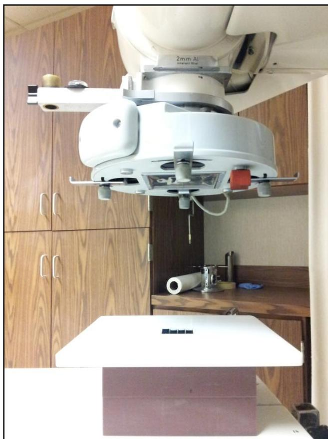
**Figure 13. PRESAGE<sup>®</sup> cuvette setup at orthovoltage unit for calibration**
