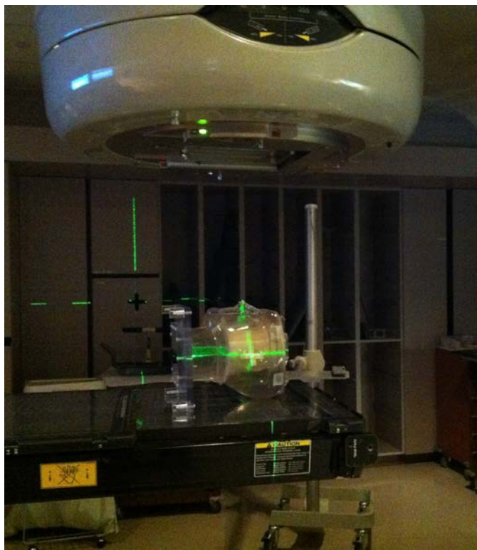
Figure 4-4: Phantom setup with laser alignment to BBs
