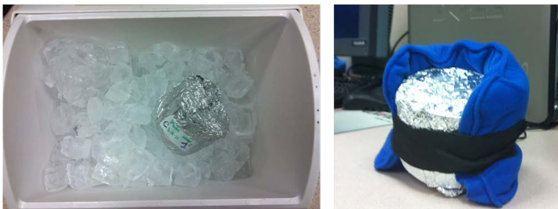
Figure 3-5: Dosimeters being brought to extreme cold or hot for irradiation. The equilibration was done in a water bath for irradiation.
