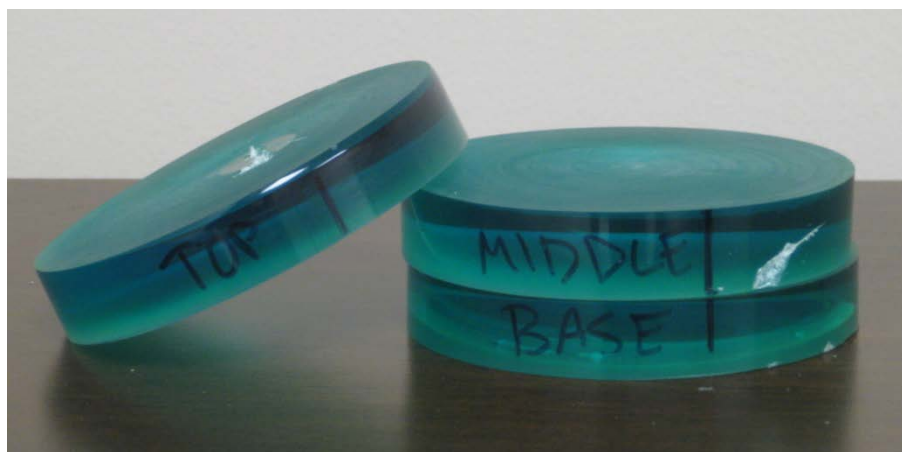
Figure 3-1: The film phantom for dose calibrations was created from a used PRESAGE ® dosimeter. Film was sandwiched between the two levels and compared to a dosimeter from the batch of PRESAGE ® being calibrated.
