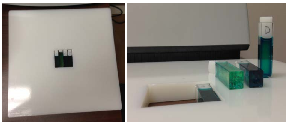
Figure 3-3: The high-impact phantom containing a cuvette cutout (left) with cuvettes inserted. A close up of the cuvettes is shown on the right.
