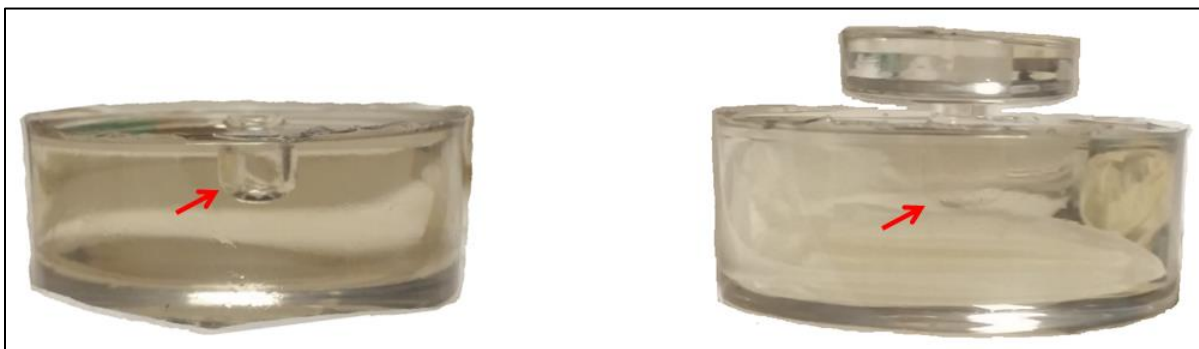
Figure 16: A side view at the dosimeter with no plug inserted (left) and with plug inserted in the cavity (right).
