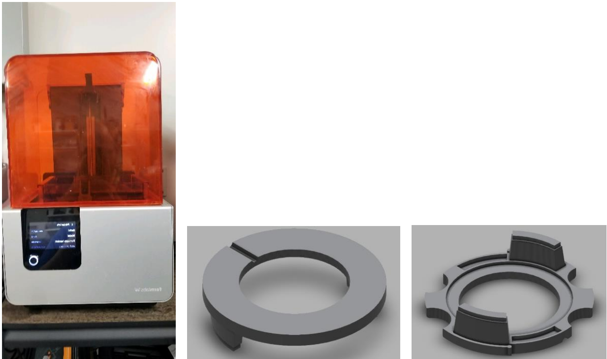
Fig. 3.8 (a) 3D printer (b) Design of top part of electrode pillar (c) Design of bottom part of electrode pillar
