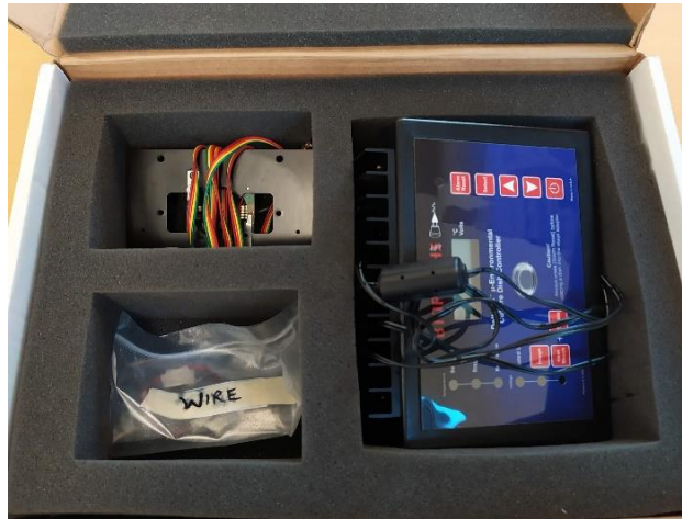
Fig. 3.13 Biopetechs temperature controller
