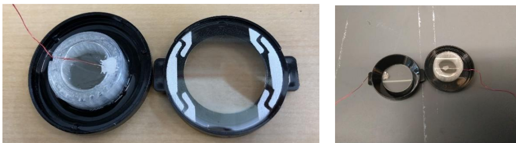
Fig. 3.12 (a) Electrode support with wire attached electrode fixed to the top cover of Delta T culture dish (b) Lab made device prototype
