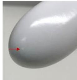
Figure 28: Small bubble formed on the tip of the rigid endorectal coil post 70 HLD cycles in the trophon<sup>®</sup> 2
