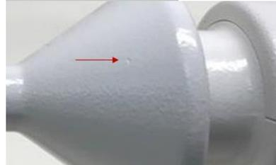
Figure 29: Chip on the base of the neck—present pre and post 100 HLD cycles.
