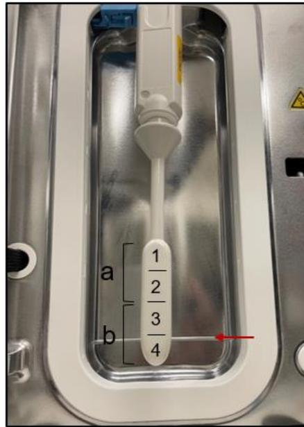
Figure 8: Arrow indicating the line that ultrasound transducers are recommended not to pass for disinfection; however, the rigid endorectal coil is longer. Locations labelled 1, 2, 3, and 4 represent the area for which each inoculated sample was placed. *Plate a* represents bacteria in locations 1 and 2, while *Plate b* represent locations 3 and 4. A syringe was used to inoculate the coil, and an L-spreader was used to spread the bacteria on the coil.
