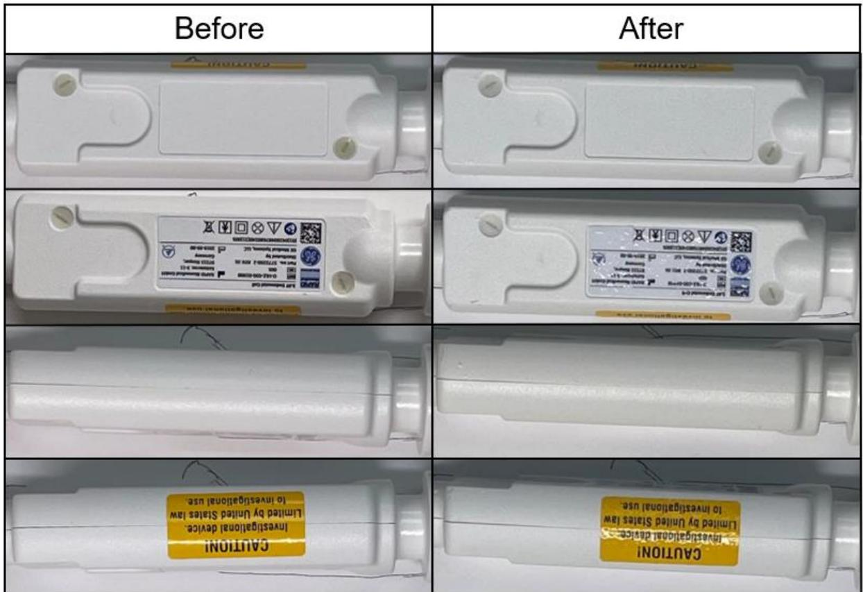
Figure 31: Images of the electronics region of the coil pre and post 100 trophon® 2 HLD cycles
