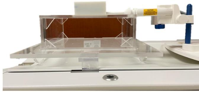
Figure 4: Acrylic stand positioned on the MRI table. Reproducible setup ensured with consistent stand placement; the stand interfaces where a head coil is placed for patient imaging and is secured closest to the coil's base. The 3D printed structure is placed atop the stand, secured in place with a recess of acrylic.
