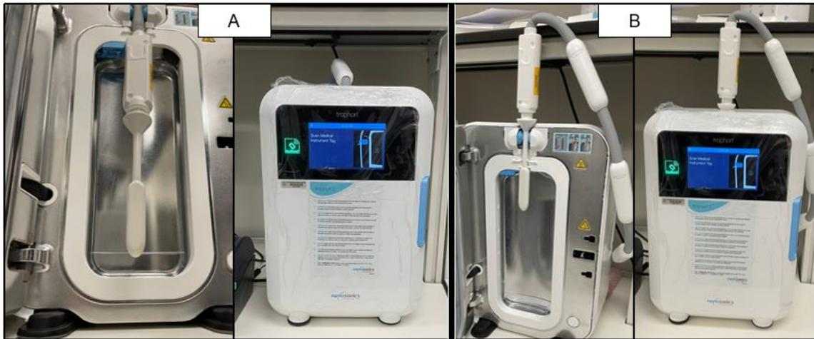
Figure 11: Two options of rigid endorectal coil placement within the trophon® 2. Setup A requires the electronic casing to receive HLD—however, the electronic casing does not require HLD and may not be sealed as sufficiently as the coil and neck of the coil; setup B fails to provide HLD to the neck of the rigid endorectal coil. Because of this, this study uses setup A for HLD of the rigid endorectal coil
