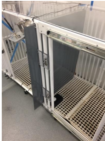
Figure 2. Opaque divider experimental setup. Two animals cooperate for food with an opaque divider between them, which prevents them from seeing each other.
